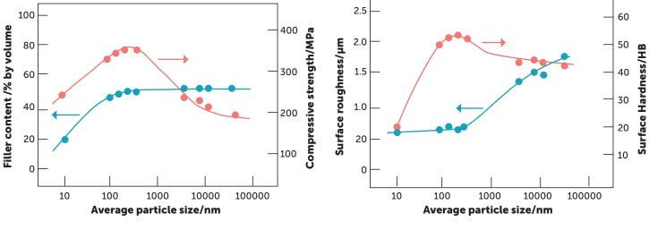
Fig. 9 Correlation between particle size, filler content, and compressive strength
