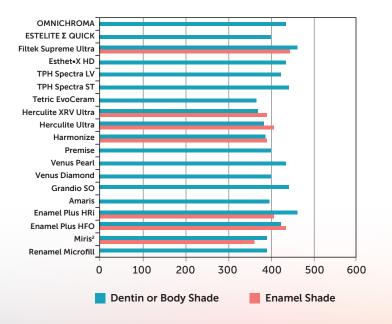
Fig. 21 Compressive strength (MPa)
