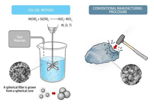
Fig. 8 Sol-Gel Method vs conventional filler method
