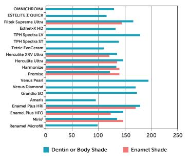
Fig. 20 Flexural strength (MPa)
