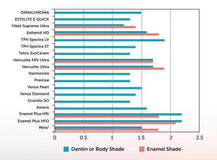
Fig. 25 Polymerization shrinkage (% linear)
