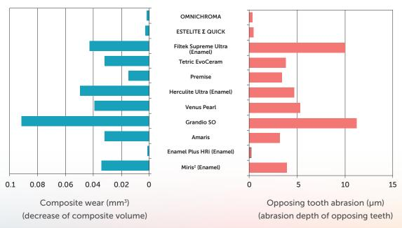
Fig. 23 Wear resistance (50,000 cycles)
