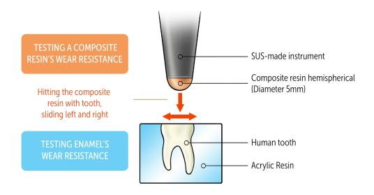
Fig. 22 Method of testing wear resistance
