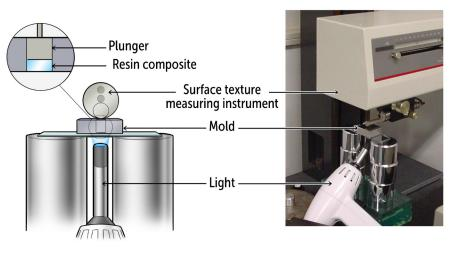
Fig. 24 Method of measuring polymerization shrinkage
