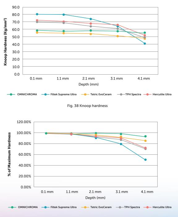
Fig. 39 Hardness top to bottom
